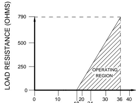
$V_{MIN} = 12 + [0.022 \times (R_{LOAD} + 300)]$
